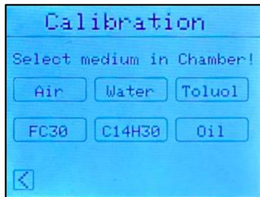
With the selection, the calibration to this medium starts. Afterwards, the second medium can be selected, in the example shown below this is water and toluene.
