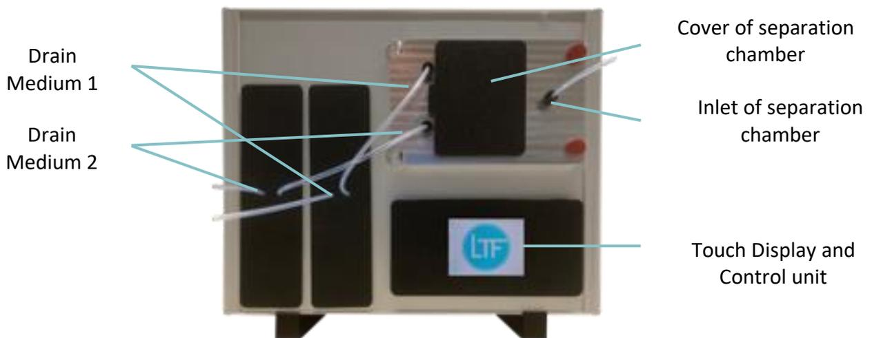
The phase separator is controlled via the touch display.
