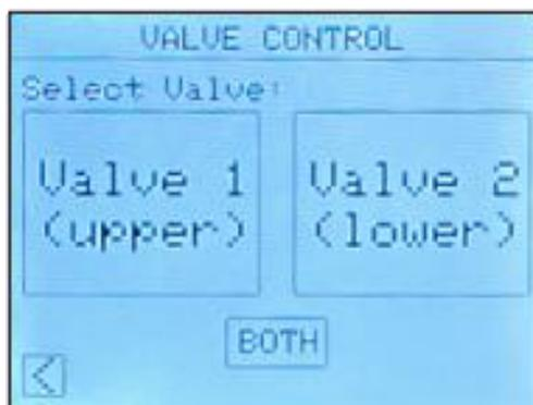
The next step is to fill the chamber with one of the media to be separated. **Via VALVE CONTROL** the menus as described under 5.2 are available here for the filling process.
